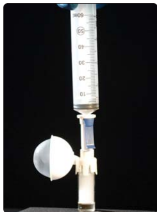
Figure 1. PhaSeal with no release of titanium smoke.
