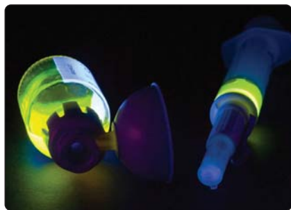
Figure 6. PhaSeal with no release of fluorescein.
