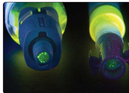
Figure 8. OnGuard Tevadaptor system with release of fluorescein droplets.
