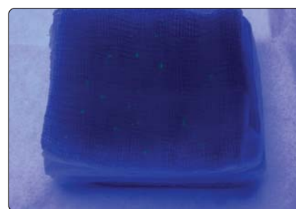
Figure 11. Alaris Smart Site touch test results show fluorescein exposure.
