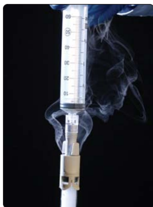
Figure 2. OnGuard Tevadaptor with release of titanium smoke.
